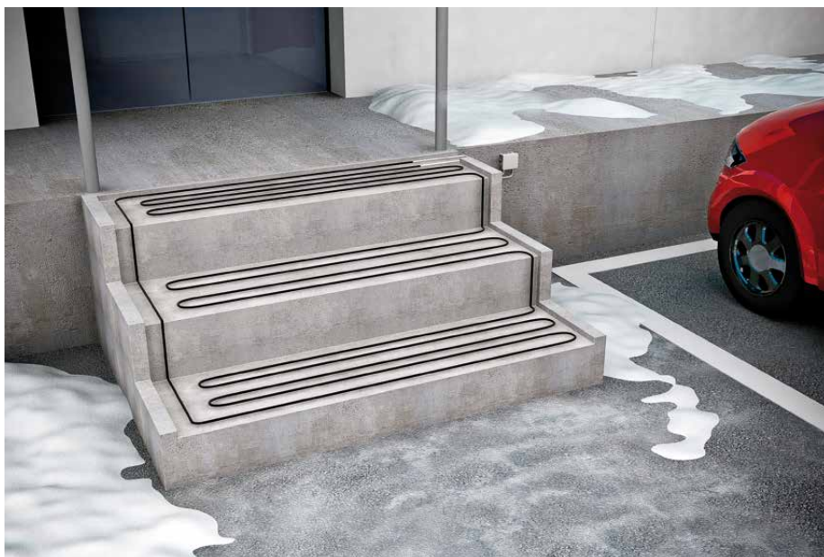
Tash is a constant wattage cable that is suitable for applications of various shapes and also for large areas. The Tash cable is always installed as a loop and both ends are connected to a junction box with a cold lead. (THE PICTURE IS AN APPROXIMATION)
